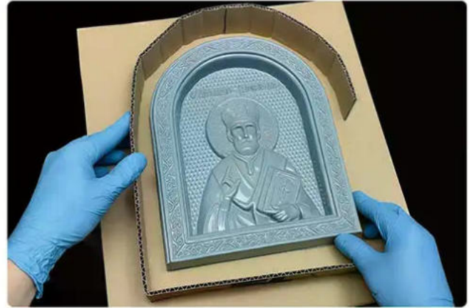
2. Build the Mold Box
