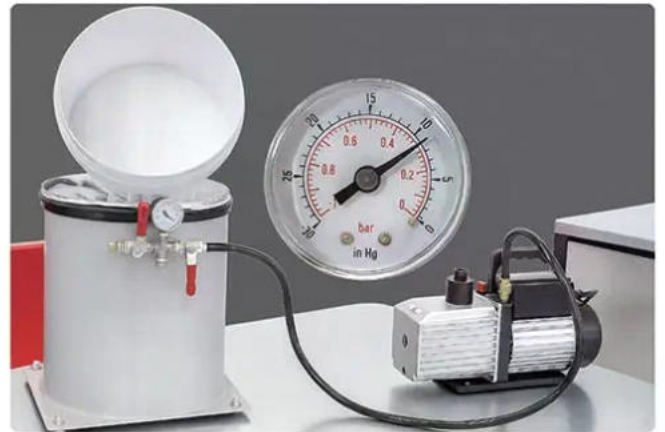
4. Vacuum Degas the Silicone
