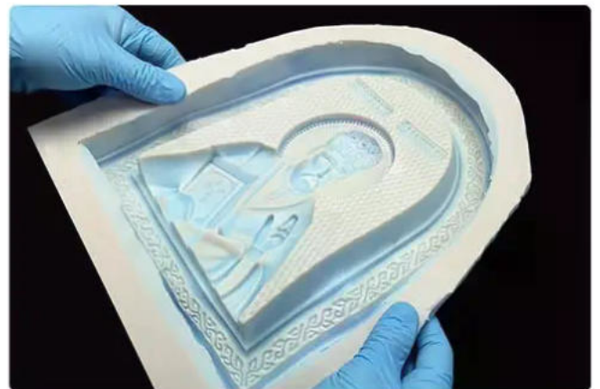
6. Cure and Demold
