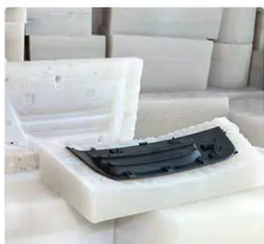
Thin Wall Enclosure Casting 薄壁外殼灌注
